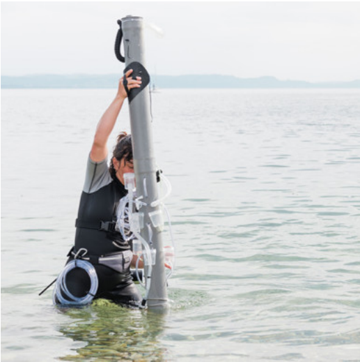
AquaQuaz™ FILTRATION MECHANIC CORE measuring tool (with stability float). 4880g, 10x20x160cm. Core sampling with good results in only 3 minutes of continued use on a 100x100x70cm zone. Control settings : analysis speed, filtering and timer. Firmly hold the Control and Stab handles and proceed to sample with continuous circular motions. Analysis results after 20 minutes out of the water.
